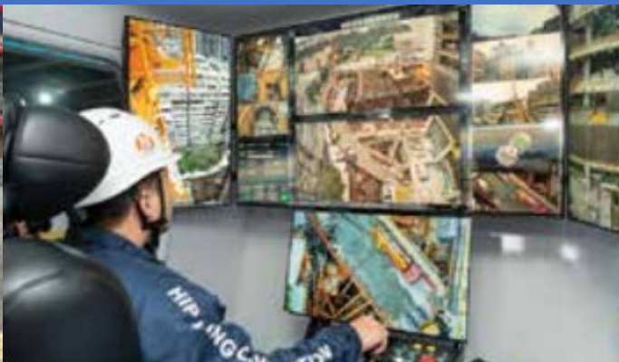
Self-Developed Distant Tower Crane Control System
