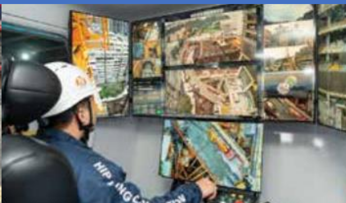
Self-Developed Distant Tower Crane Control System
